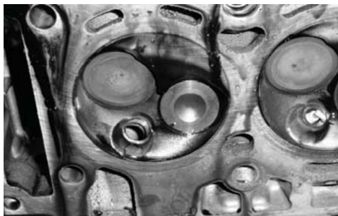
Fig. 1. Simulated damage of exhaust valve
